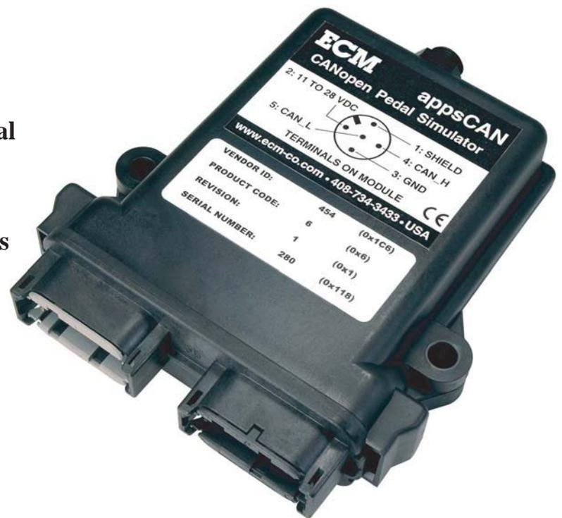
Most vehicles sold today do not have a direct physical connection between the accelerator pedal and the engine's throttle. Instead, command signals from the accelerator pedal are sent to the engine controller and the engine's throttle is controlled by an electric motor. When engines or vehicles are tested in dynamometer cells, it is no longer necessary to have a robot or actuator pushing on the accelerator pedal if these signals can be simulated.
